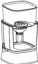
4) Put the upper barrel with filter on the support base.
