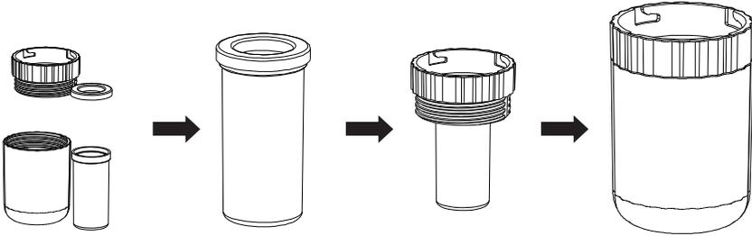
1) Filter housing, seal ring and filter.
