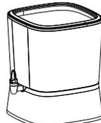
3) Put the support base on the upper barrel.
