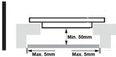
There are ventilation holes around outside of the hob. YOU MUST ensure these holes are not blocked by the worktop when you put the hob into position.
